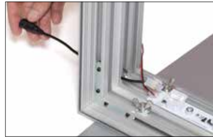
3 Insert the adaptor cable in the hole in the profile. Each hole fits 2 cables.
