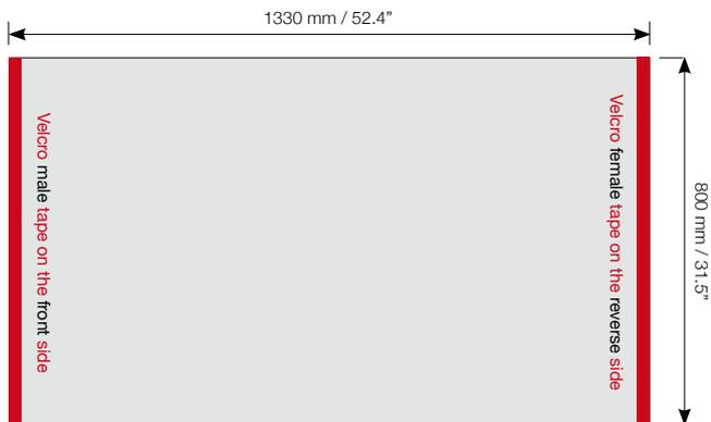
Attach a 20 mm Velcro male tape on the front side and a female on the other edge on the reverse side.
