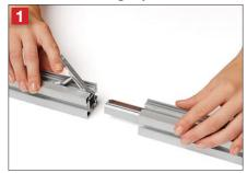
Lift the FASTclamp lever while inserting the profile stem. Make sure that the small metal bracket is in direct contact with the FASTclamp.
