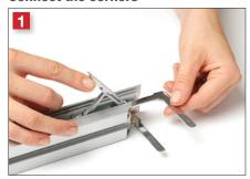
Lift FASTclamp lever and fully insert the 90° L-bracket. Lock clamp by pressing lever back down into the channel. Repeat for both clamps on this frame profile.
