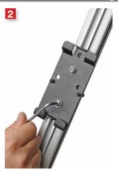
Use an allen key to lock in place with the screws.
