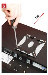
Attach the two connection rails to the screen, taking note to properly orient with the top of screen.
