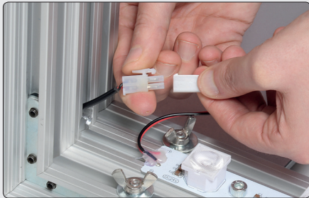
4 Connect the contacts from the LED-bar to the adaptor cable.
