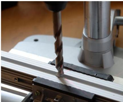
**1** Drill a 13 mm hole in the center of that profile you want to insert a Twist Lock.
