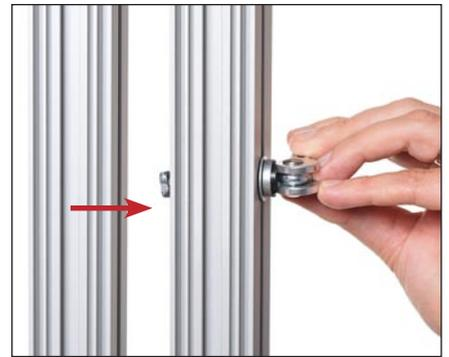
**3** Bring the second profile/frame into contact with the clamp pin. Holding the clamp handle perpendicular to the profile will provide proper pin alignment.
